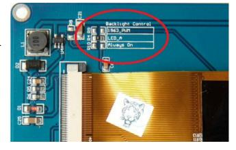
pads marked "1963-PWM". The Armmite F4 can then control the brightness via the SSD1963 controller.
